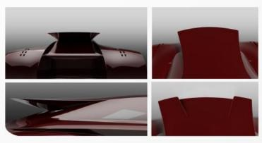
The spoiler can be divided in 3 parts. The middle part regulate the drag and enhance the aerodynamic brake. The two sides parts can improve the lateral downforce when it is needed.
